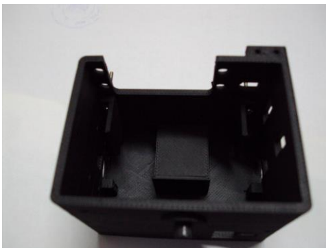
5. actual shell with battery brackets
